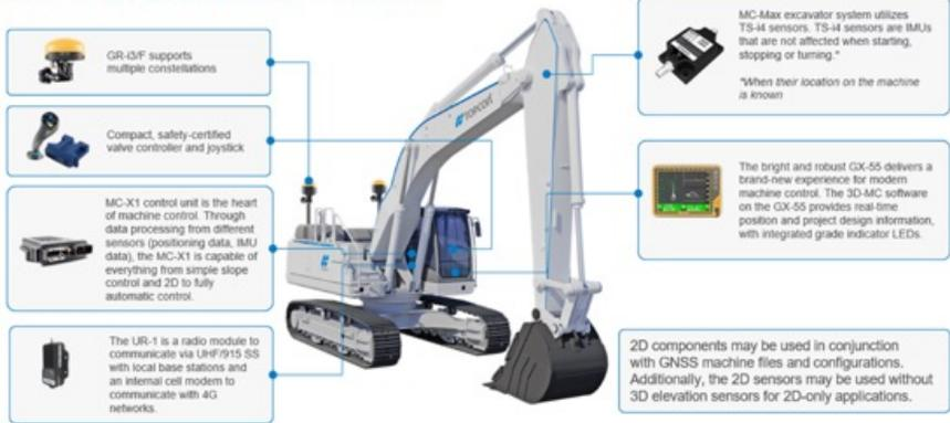
*Figure 2: Example of a machine being equipped with GNSS machine control systems.*
